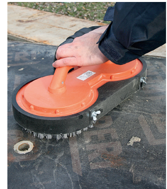
Cleaning formwork units
