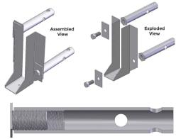
Double threaded cylinder bolt assembled
