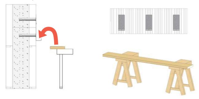
Check ledger bracket for correct height and level Chalk line
