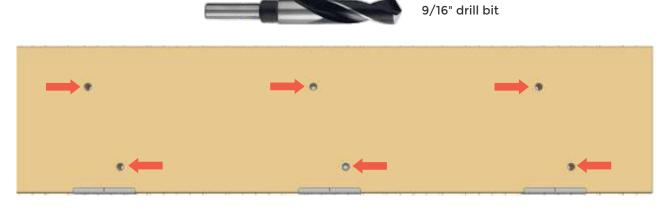
Bolt the ledger board to the BURMON-ICFWL using the Hex Head bolts and washers supplied. Tighten securely.
